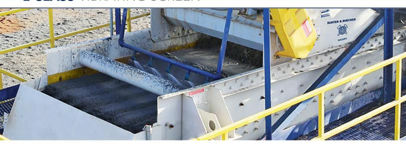
The Niagara L-Class vibrating screen is a versatile and easy to maintain linear machine, with no timing belts or gears that need replacing.
